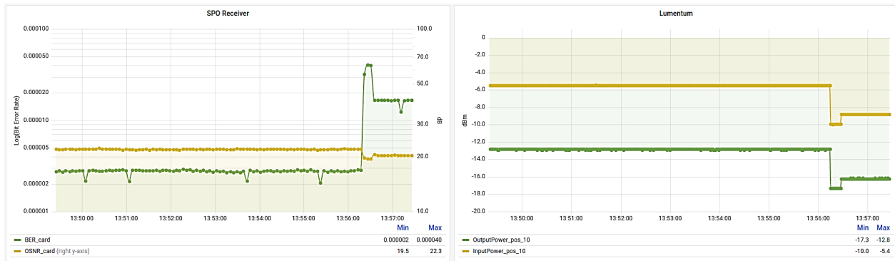
Fig. 10. Test 2 (TX power reduction): Grafana P2PT monitors at A1 agent, showing failure and recovery events.
